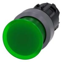
Illuminated mushroom pushbutton, 22 mm, round, plastic with metal front ring, green, 30 mm, momentary contact type, with laser labeling, upper case
