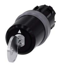
Key-operated switch BKS, 22 mm, round, plastic with metal front ring, lock number S1, with 2 keys, 3 switch positions I-O-II, latching, actuating angle  $2x45^{\circ},\,10:30h/12h/13:30h,$  Key removal I+II, with laser labeling, lower case
