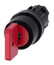
Key-operated switch O.M.R, 22 mm, round, plastic, lock number 73037, red, with 2 keys, 3 switch positions I-O-II, latching, actuating angle 2x45°, 10:30h/12h/13:30h, key removal O+I, with laser labeling, inscription or symbol Customer-specific selection with SIRIUS ACT configurator (CIN)
