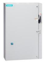
Non-reversing motor starter, Size 3, Three phase full voltage, Solid-state overload relay, OLR amp range 25-100A, Combination type, 200A fusible disconnect, 200A/250V fuse clip, Enclosure NEMA type 1, Indoor general purpose use, Extra-wide enclosure
