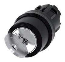
RONIS key-operated switch, 22 mm, round, plastic, special lock, with 2 keys, 2 switch positions O-I, latching, actuating angle  $90^\circ$ , 10:30h/13:30h, key removal O+I, possible special locks: SB31, 421, 455
