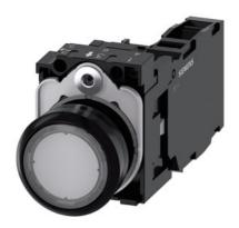
Illuminated pushbutton, 22 mm, round, plastic, clear, pushbutton, flat, momentary contact type, with holder, 1 NO+1 NC, LED module with integrated LED 110 V AC, screw terminal, Z=20-unit packaging
