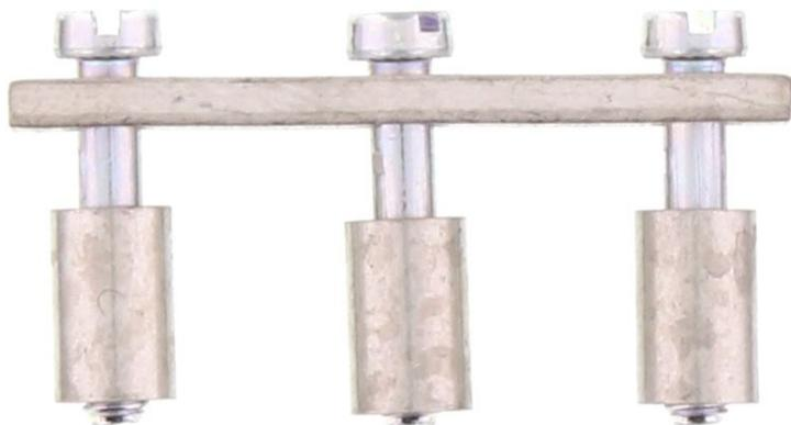
Cross-connector, No. of poles: 3, Mounting type: Can be screwed on, Width: 32 mm, Rated cross-section: 16 mm<sup>2</sup>, Colour: natural
