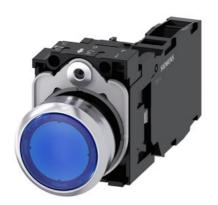
Illuminated pushbutton, 22 mm, round, metal, shiny, blue, pushbutton, flat, momentary contact type, with holder, 1 NO+1 NC, LED module with integrated LED 24 V AC/DC, screw terminal, Z=20-unit packaging
