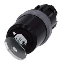
Key-operated switch BKS, 22 mm, round, plastic with metal front ring, lock No. E9 (VW), without key, 2 switch positions O-I, latching, actuating angle 90°, 10:30h/13:30h, key removal O, with laser labeling, upper case and lower case, always upper case at the beginning of the word
