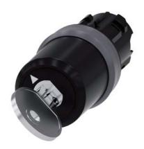
Key-operated switch BKS, 22 mm, round, plastic with metal front ring, Lock No. E2 (VW), without key, 2 switch positions O-I, latching, actuating angle 90°, 10:30h/13:30h, key removal O+I, with laser labeling, upper case and lower case, always upper case at the beginning of the word
