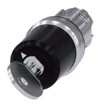
Key-operated switch BKS, 22 mm, round, metal, shiny, lock number S1, with 2 keys, 2 switch positions O-I, latching, actuating angle 90°, 10:30h/13:30h, key removal I, with laser labeling, upper case and lower case, always upper case at the beginning of the word
