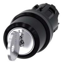
RONIS key-operated switch, 22 mm, round, plastic, lock number SB30, with 2 keys, 3 switch positions I>O<II, momentary contact on the left, latching on the right, actuating angle 2x45°, 10:30h/12h/13:30h, key removal O, possible special locks: SB31, 421, 455 Z=50-unit packaging
