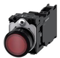
Illuminated pushbutton, 22 mm, round, plastic, red, pushbutton, flat, momentary contact type, with holder, 1 NO+1 NC, LED module with integrated LED 24 V AC/DC, spring-type terminal, with laser labeling, upper case and lower case, always upper case at beginning of line
