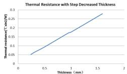
\*Specimen Area: 1inch2 Rate of strain= 1.0mm/min \*Specimen Area: 1inch<sup>2</sup> The thickness of sample is controled by limit Decreased Thickness step = 0.1mm
