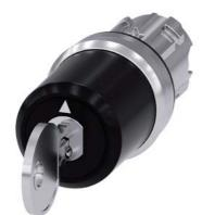
key-operated switch Siemens, 22 mm, round, metal, shiny, lock number SSG10, with 2 keys, 3 switch positions I-O<II, left latching, momentary contact type on the right, actuating angle 2x45°, 10:30h/12h/13:30h, key removal O, with laser labeling, upper case and lower case, always upper case at beginning of line
