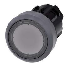
Illuminated pushbutton, 22 mm, round, plastic with metal front ring, clear, pushbutton, flat, latching, Push-to-release mechanism, with laser labeling, lower case
