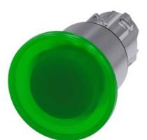
Illuminated mushroom pushbutton, 22 mm, round, metal, shiny, green, 40 mm, 3 switch positions, latches after pushing in, unlatches by pull-tounlatch mechanism to center position, after pulling out the button Retraction to center position, with laser labeling, upper case and lower case, always upper case at beginning of line
