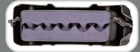
Air pockets between the two walls provide superior shock and impact protection
