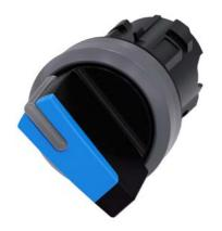
Selector switch, illuminable, 22 mm, round, plastic with metal front ring, blue, selector switch, short, 2 switch positions O-I, latching, actuating angle  $90^{\circ}$ , 10:30h/13:30h, with laser labeling, lower case
