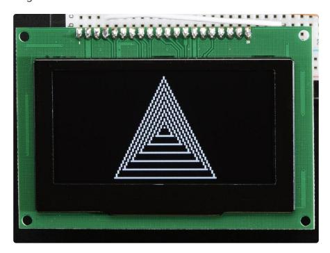
The power requirements depend a little on how much of the display is lit but on average the display uses about 50-150mA from the 3.3V supply. Built into the OLED driver is a simple switch-cap charge pump that turns 3.3V into a high voltage drive for the OLEDs.
