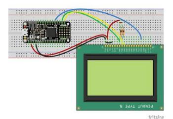
OLED Pin #1 to Microcontroller GND
