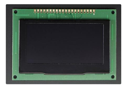
The pins on these modules are not well marked, but the one on left is #1 and the pins increment in order until the one on the very right, #20
