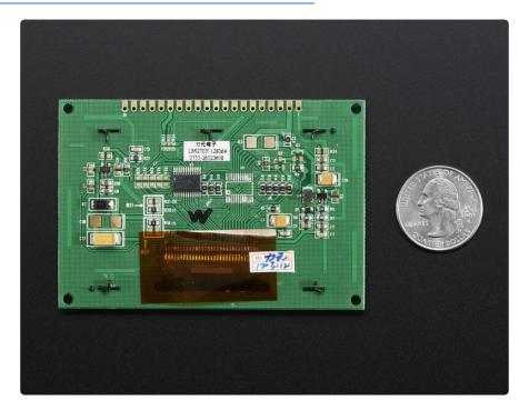
Getting started is easy! We have a detailed tutorial and example code in the form of an Arduino library for text and graphics. () You'll need a microcontroller with more than 1K of RAM since the display must be buffered. The library can print text, bitmaps, pixels, rectangles, circles and lines. It uses 1K of RAM since it needs to buffer the entire display but its very fast! The code is simple to adapt to any other microcontroller.
