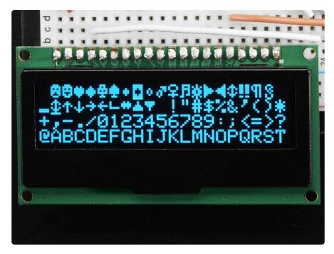
The Adafruit\_GFX library for Arduino provides a common syntax and set of graphics functions for all of our TFT, LCD and OLED displays. This allows Arduino sketches to easily be adapted between display types with minimal fuss...and any new features, performance improvements and bug fixes will immediately apply across our complete offering of displays.
