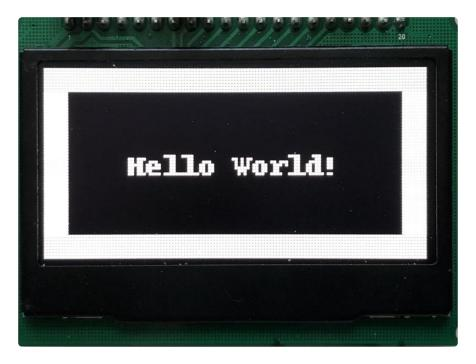
If you have the 2.3" 128x32 OLED Display, here's what the final output looks like with the height set to 32 and the border size set to 5:
