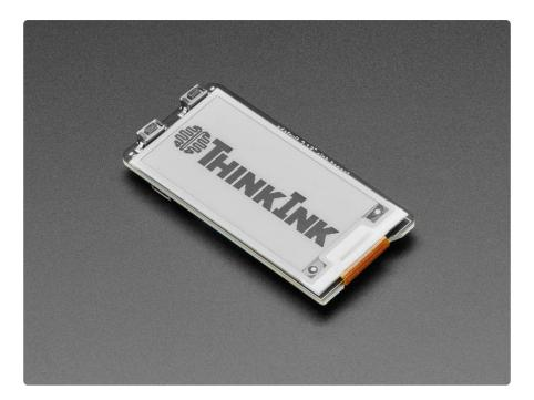
Easy e-paper finally comes to Raspberry Pi, with this bonnet that's designed to make it a breeze to add a 2.13" 250x122 crisp monochromic elnk display. Chances are you've seen one of those new-fangled 'e-readers' like the Kindle or Nook. They have gigantic electronic paper 'static' displays - that means the image stays on the display even when power is completely disconnected. The image is also high contrast and very daylight readable. It really does look just like printed paper!
