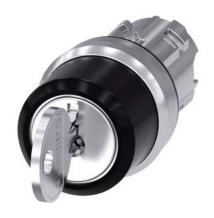
RONIS key-operated switch, 22 mm, round, metal, shiny, lock number SB30, with 2 keys, 3 switch positions I-O-II, latching, actuating angle 2x45°, 10:30h/12h/13:30h, key removal O+I, possible special locks: SB31, 421, 455, with laser labeling, inscription or symbol Customer-specific selection with SIRIUS ACT configurator (CIN)
