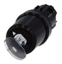
Key-operated switch BKS, 22 mm, round, plastic, Lock No. E2 (VW), without key, 2 switch positions O-I, latching, actuating angle 90°, 10:30h/13:30h, key removal O+I, with laser labeling, lower case
