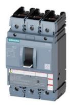
circuit breaker 3VA5 UL frame 250 breaking capacity class M 35kA @ 480 V 3-pole, line protection TM230, FTAM, In=110A overload protection Ir=110A fixed short-circuit protection Ii=5...10 x In UL489 SB (naval), 50 deg. cel. cable connection on both sides
