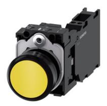
Pushbutton, 22 mm, round, plastic, yellow, pushbutton, flat, momentary contact type, with holder 1 NO+1 NC, spring-type terminal, with laser labeling, lower case
