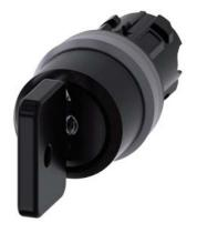
Key-operated switch O.M.R, 22 mm, round, plastic with metal front ring, lock number 73034, black, with 2 keys, 3 switch positions I-O<II, left latching, right momentary contact type, actuating angle 2x45°, 10:30h/12h/13:30h, key removal I, with laser labeling, inscription or symbol Customer-specific selection with SIRIUS ACT configurator (CIN)
