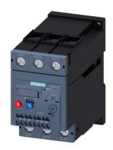
Overload relay 54...65 A Thermal For motor protection Size S2, Class 10 Stand-alone installation Main circuit: Screw Auxiliary circuit: spring-type terminal Manual-Automatic-Reset
