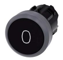
Pushbutton, 22 mm, round, plastic with metal front ring, black, inscription: O, pushbutton, flat momentary contact type, Z=100-unit packaging
