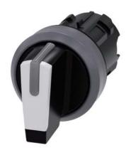
Selector switch, illuminable, 22 mm, round, plastic with metal front ring, white, selector switch, short, 3 switch positions I-O-II, latching, actuating angle  $2x45^{\circ}$ , 10:30h/12h/13:30h, with laser labeling, upper case and lower case, always upper case at the beginning of the word
