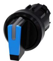
Selector switch, illuminable, 22 mm, round, plastic, blue, selector switch, short, 3 switch positions I-O-II, latching, actuating angle  $2x45^{\circ}$ , 10:30h/12h/13:30h Z=50-unit packaging
