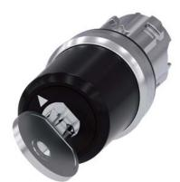
Key-operated switch BKS, 22 mm, round, metal, shiny, Lock No. E9 (VW), without key, 2 switch positions O-I, latching, actuating angle 90°, 10:30h/13:30h, key removal O+I, with laser labeling, upper case and lower case, always upper case at beginning of line
