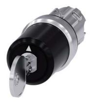
Key-operated switch BKS, 22 mm, round, metal, shiny, lock number S1, with 2 keys, 3 switch positions I-O-II, latching, actuating angle  $2x45^{\circ}$ , 10:30h/12h/13:30h, Key removal I+O+II, with laser labeling, upper case and lower case, always upper case at the beginning of the word
