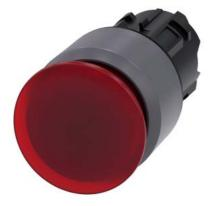
Illuminated mushroom pushbutton, 22 mm, round, plastic with metal front ring, red, 30 mm, latching, pull-to-unlatch mechanism, with laser labeling, upper case and lower case, always upper case at beginning of line
