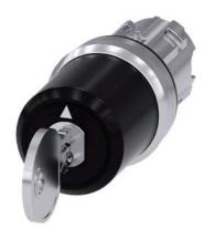
Key-operated switch BKS, 22 mm, round, metal, shiny, lock number S1, with 2 keys, 3 switch positions I-O<II, left latching, right momentary contact type, actuating angle 2x45°, 10:30h/12h/13:30h, key removal I, with laser labeling, lower case
