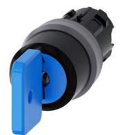
Key-operated switch O.M.R, 22 mm, round, plastic with metal front ring, lock number 73038, blue, with 2 keys, 3 switch positions I-O-II, latching, actuating angle 2x45°, 10:30h/12h/13:30h, key removal O, with laser labeling, upper case and lower case, always upper case at the beginning of the word
