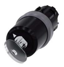
key-operated switch Siemens, 22 mm, round, plastic with metal front ring, lock number SSG10, with 2 keys, 2 switch positions O<I, momentary contact type, actuating angle 45°, 10:30h/12h, key removal O, with laser labeling, lower case
