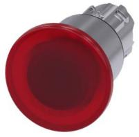
Illuminated mushroom pushbutton, 22 mm, round, metal, shiny, red, 40 mm, 3 switch positions, after pushing in Retraction to center position, after pulling out the button Retraction to center position, with laser labeling, inscription or symbol Customer-specific selection with SIRIUS ACT configurator (CIN)
