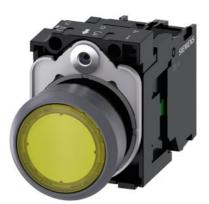
Illuminated pushbutton, 22 mm, round, plastic with metal front ring, yellow, pushbutton, flat, momentary contact type, with holder, 1NO, LED module with integrated LED 110 V AC, screw terminal, with laser labeling, upper case
