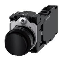
Pushbutton, 22 mm, round, plastic, black, pushbutton, raised, momentary contact type, with holder 1 NO+1 NC, screw terminal, with laser labeling, upper case
