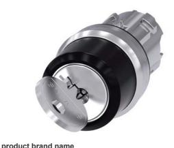
RONIS key-operated switch, 22 mm, round, metal, shiny, lock number 455, with 2 keys, 2 switch positions O-I, latching, actuating angle  $90^\circ$ , 10:30h/13:30h, key removal O, with laser labeling, upper case and lower case, always upper case at the beginning of the word
