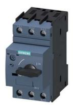
Special type Circuit breaker size S00 for motor protection, CLASS 10 A-release 2.8...4 A N release 52 A screw terminal Standard switching capacity Ambient temperature -50  $^\circ$ C 500 switching cycles
