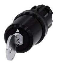
Key-operated switch BKS, 22 mm, round, plastic, lock number S1, with 2 keys, 3 switch positions I>O<II, momentary contact on the left, latching on the right, actuating angle 2x45°, 10:30h/12h/13:30h, key removal O, with laser labeling, upper case and lower case, always upper case at beginning of line
