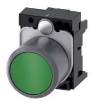
Pushbutton, compact, with extended stroke (12 mm), 22 mm, round, plastic with metal front ring, green, pushbutton, flat, momentary contact type, with holder, with laser labeling, symbol number according to, ISO 7000 or IEC 60417
