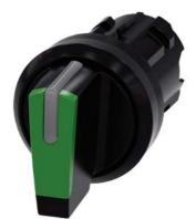
Selector switch, illuminable, 22 mm, round, plastic, green, selector switch, short, 3 switch positions I>O<II, momentary contact on the left, latching on the right, actuating angle 2x45°, 10:30h/12h/13:30h, with laser labeling, inscription or symbol Customer-specific selection with SIRIUS ACT configurator (CIN)
