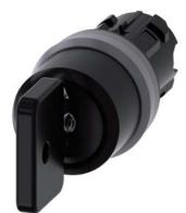
Key-operated switch O.M.R, 22 mm, round, plastic with metal front ring, lock number 73034, black, with 2 keys, 3 switch positions I-O-II, latching, actuating angle 2x45°, 10:30h/12h/13:30h, Key removal I+O+II, with laser labeling, upper case and lower case, always upper case at beginning of line
