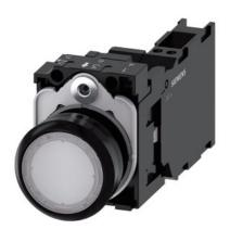
Illuminated pushbutton, 22 mm, round, plastic, white, pushbutton, flat, momentary contact type, with holder, 1 NO+1 NC, LED module with integrated LED 110 V AC, spring-type terminal, with laser labeling, symbol number according to, ISO 7000 or IEC 60417
