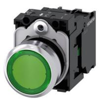
Illuminated pushbutton, 22 mm, round, Metal, shiny, green, pushbutton, flat, momentary contact type, with holder, 1NO, LED module with integrated LED 230 V AC, screw terminal, with laser labeling, lower case
