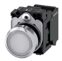
Illuminated pushbutton, 22 mm, round, metal, shiny, white, pushbutton, flat, momentary contact type, with holder, 1NO, LED module with integrated LED 24 V AC/DC, spring-type terminal, Z=20-unit packaging
