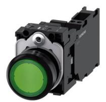
Illuminated pushbutton, 22 mm, round, plastic, green, pushbutton, flat, momentary contact type, with holder, 1 NO+1 NC, LED module with integrated LED 110 V AC, spring-type terminal, with laser labeling, lower case
